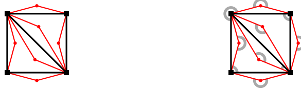
Figure 5: A planar Laman graph with a planar embedding that does not (left) and a planar embedding that does (right) admit an angle cover.
