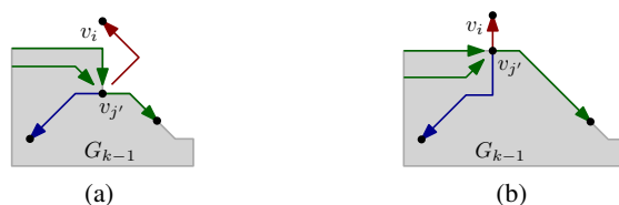
Figure 7: (a) e' = (v_{j'}, v_i) cannot be drawn bend-less. (b) Shifting v_{j'} up resolves the problem.
